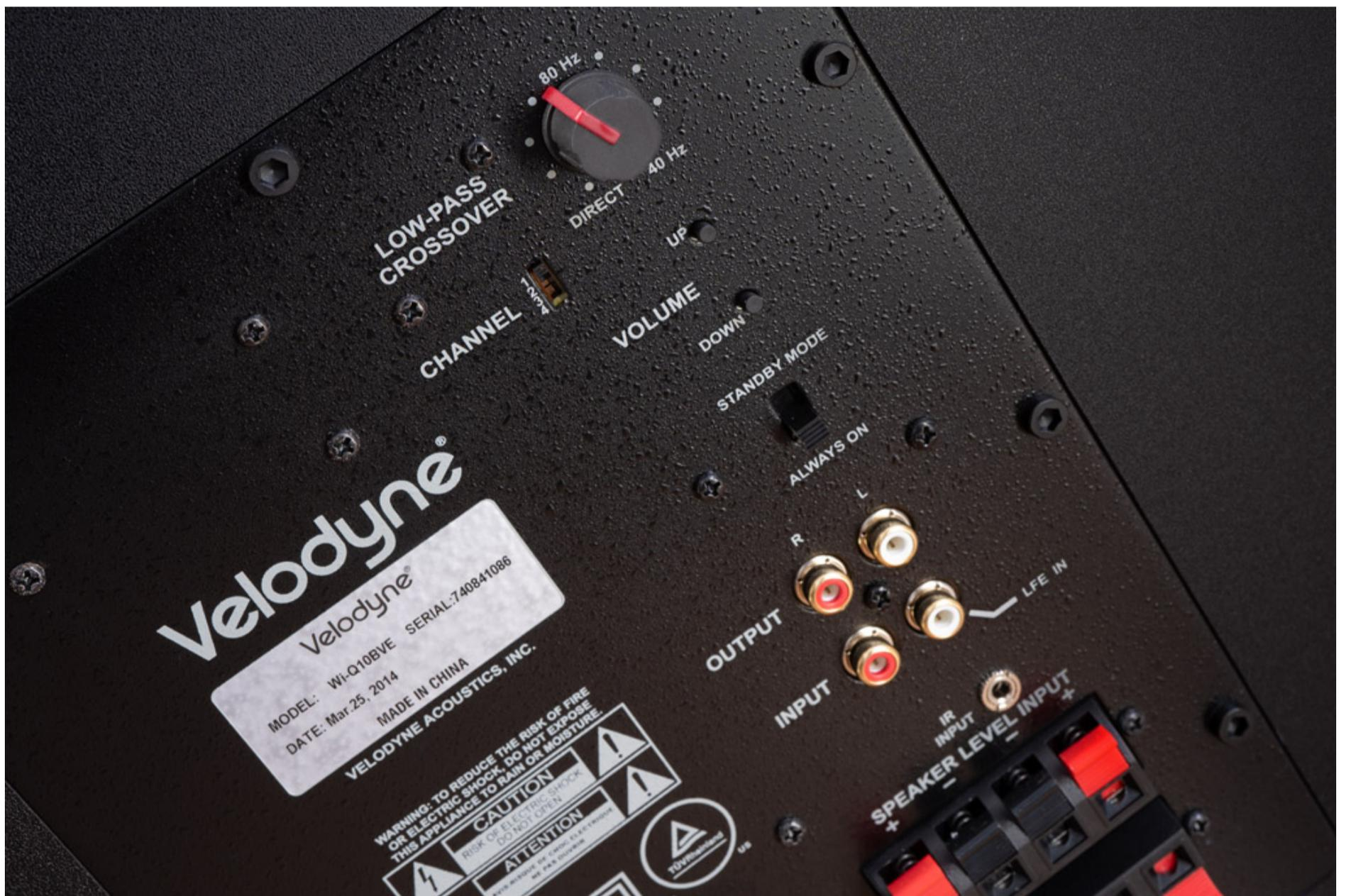
All controls, switches and sockets are located on the back of the sub. Among other things, there are also two low-level inputs. This means that the WI-Q10 can also be operated with a wired connection.
