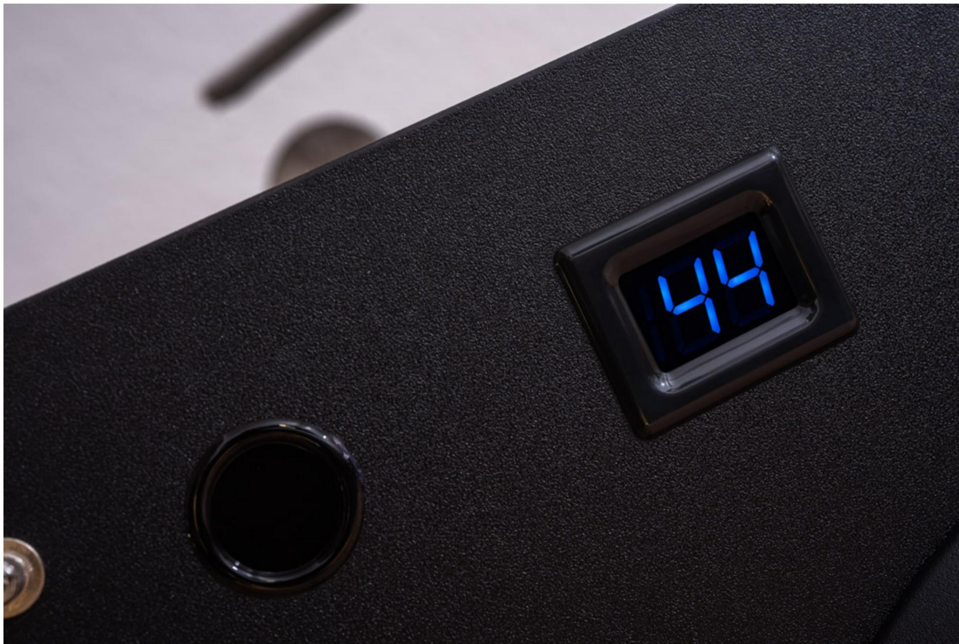
The display in the front provides information about the currently selected volume. If necessary, it can also be dimmed or switched off completely.
