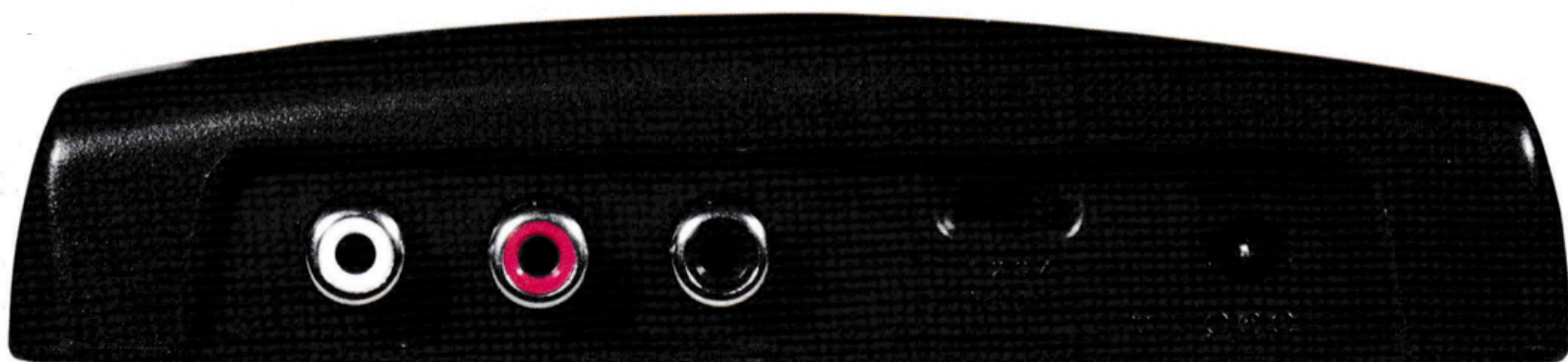
In addition to the connections for signal supply, we find a switch for channel selection. Four possible options are available. It was therefore easy to control several devices from one
